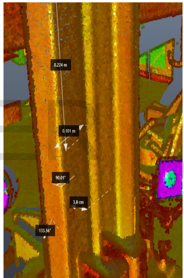
Figure 4. Using Recap Point Cloud programs to measure imperfection of specimens
